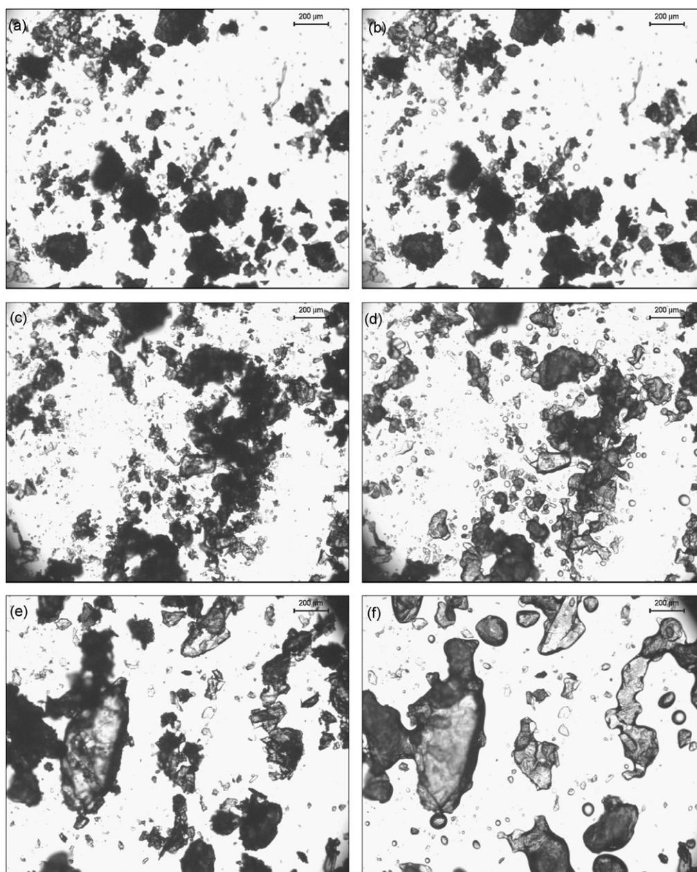
**Fig. 12.** Microscopy images of the system myristic acid (4) + stearic acid (6). (a and b)  $x_4 \cong 0.50$ ; (c and d)  $x_4 \cong 0.55$ ; (e and f)  $x_4 \cong 0.60$ ; the left column at 318.15 K and right column at 322.15 K.
