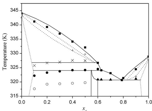
Fig. 15. Phase diagram of the system myristic acid (4)+stearic acid (6). (■) Fusion temperature; (●) peritectic temperature; (▲) eutectic temperature; (×) metatectic temperature; (+, ○) transitions temperatures on the solid phase; (Δ) transition on the solid phase of the pure component.
