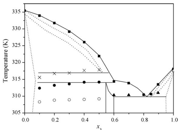
Fig. 14. Phase diagram of the system lauric acid (3)+palmitic acid (5). (■) Fusion temperature; (●) peritectic temperature; (▲) eutectic temperature; (×) metatectic temperature; (○) transition temperature on the solid phase; (Δ) transition on the solid phase of the pure component.
