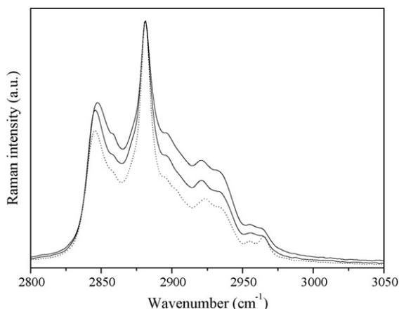
**Fig. 6.** FT-Raman spectra for myristic acid (4) + stearic acid (6) system at 322.15 K in the range 2800–3050  $\text{cm}^{-1}$ . Dashed line represents the sample ( $x_4 \cong 0.50$ ) before melting; from top to bottom:  $x_4 \cong 0.55$ ,  $x_4 \cong 0.50$ .
