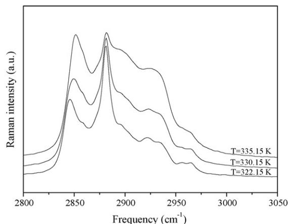
**Fig. 7.** FT-Raman spectra for myristic acid (4) + stearic acid (6) system at  $x_4 \cong 0.30$  in the range 2800–3050  $\text{cm}^{-1}$ .
