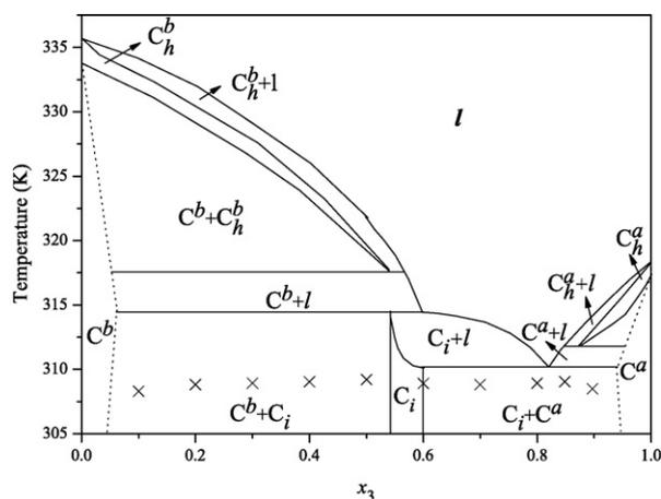
**Fig. 1.** Global phase diagram for the fatty acids systems studied in this work.  $C$  solid solution formed on the extremes of the phase diagram rich in one of the components of the mixture;  $C_i$  solid solution formed by the mixture of the components;  $C_h$  solid phase formed after the metatectic reaction;  $l$  liquid phase;  $\times$  transition on the solid phase. The superscript  $a$  and  $b$  represents the components of the mixture.
