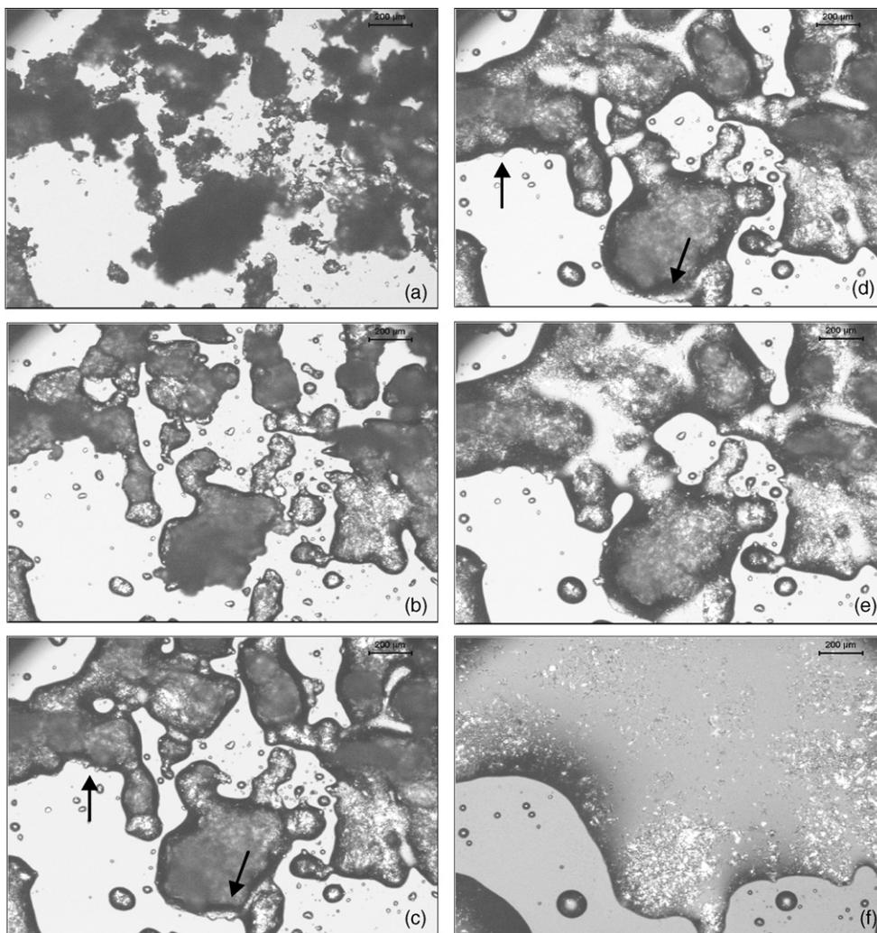
**Fig. 10.** Microscopy images of the system myristic acid (4) + stearic acid (6) + at  $x_4 \cong 0.50$ . (a)  $323.15$  K; (b)  $325.15$  K; (c)  $326.15$  K; (d)  $326.65$  K; (e)  $327.15$  K; and (f)  $331.15$  K.
