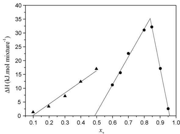
**Fig. 3.** Tamman plot for capric acid (2) + myristic acid (4) system. (▲) Enthalpy of the peritectic reaction; (●) enthalpy of the eutectic reaction; (—) fitting to the experimental results obtained.
