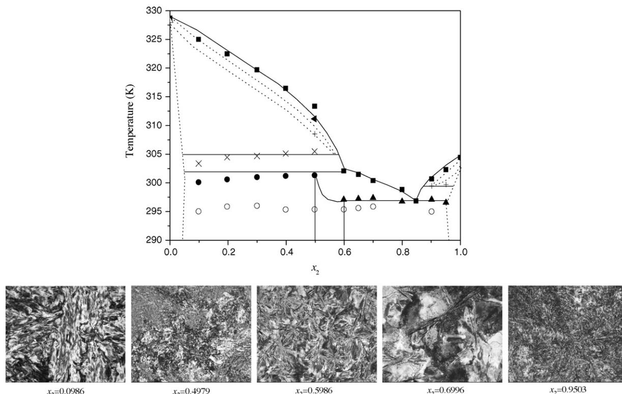
**Fig. 11.** Phase diagram of the system capric acid (2) + myristic acid (4) and images of this system. (■) Fusion temperature; (●) peritectic temperature; (▲) eutectic temperature; (×) metatectic temperature; (+, ○, ◀) transitions temperatures on the solid phase; (△) transition on the solid phase of the pure component.
