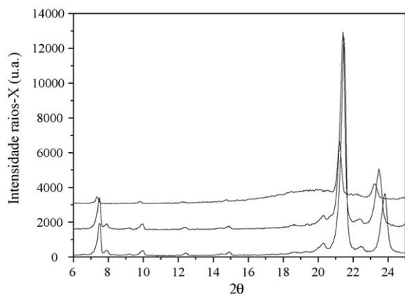
**Fig. 9.** X-ray powder diffraction patterns for the system myristic acid (4) + stearic acid (6) at constant composition  $x_4 \cong 0.65$ . From top to bottom:  $T = 322.15$  K,  $T = 318.15$  K and  $303.15$  K.
