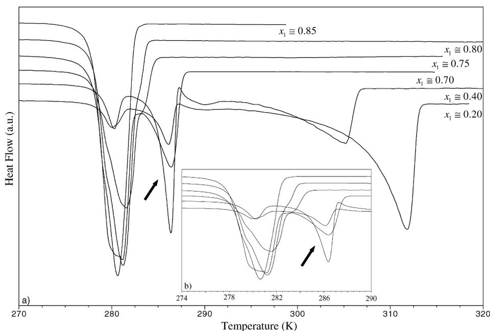
**Fig. 2.** (a) Thermograms for the system caprylic acid (1) + lauric acid (2); (b) inset of the thermograms around the peritectic and eutectic transition.
