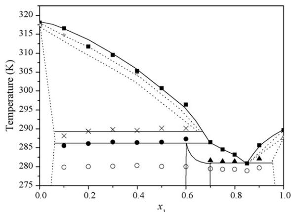
Fig. 13. Phase diagram of the system caprylic acid (1)+lauric acid (3). (■) Fusion temperature; (●) peritectic temperature; (▲) eutectic temperature; (×) metatectic temperature; (+, ○) transitions temperatures on the solid phase; (Δ) transition on the solid phase of the pure component.
