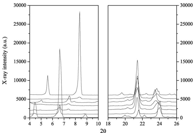
**Fig. 8.** X-ray powder diffraction patterns for the system myristic acid (4) + stearic acid (6). From top to bottom:  $x_4 = 1.00$ ,  $x_4 \cong 0.95$ ,  $x_4 \cong 0.65$ ,  $x_4 \cong 0.55$ ,  $x_4 \cong 0.25$ ,  $x_4 \cong 0.05$  and  $x_4 = 0.00$ ; (a) range  $4^\circ \leq 2\theta \leq 10^\circ$ ; (b) range  $18^\circ \leq 2\theta \leq 26^\circ$ .
