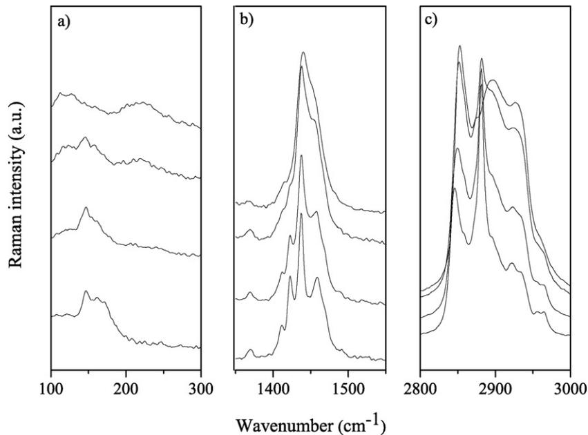
**Fig. 4.** Temperature dependence of the FT-Raman spectra for myristic acid (4)+stearic acid (6) system at  $x_4 \cong 0.25$ : (a) range 100–300  $\text{cm}^{-1}$ ; (b) range 1350–1550  $\text{cm}^{-1}$ ; (c) range 2800–3000  $\text{cm}^{-1}$ . From bottom to top: 318.4, 322.15, 328.15 and 343.15 K.
