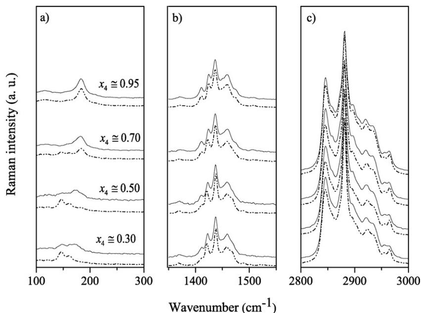
**Fig. 5.** FT-Raman spectra for myristic acid (4)+stearic acid (6) system at 313.15 K. The dashed lines represent the spectra before melting and the solid lines after melting. The compositions for (b) and (c) are the same presented in (a).
