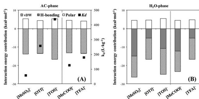
**Fig. 9** Predicted COSMO-RS contributions to interaction energies of (A) IL-AC and (B) IL-water for  $[C_4C_1\text{im}]^+$  based ILs with different anions.
