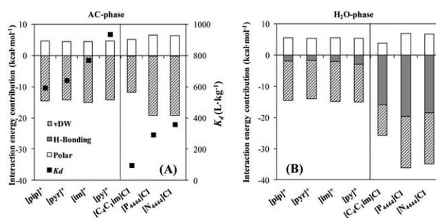
**Fig. 7** Predicted COSMO-RS contributions to interaction energies of (A) IL-AC and (B) IL-water for [NTf<sub>2</sub>]<sup>-</sup> and Cl<sup>-</sup>-based ILs with different cation families.
