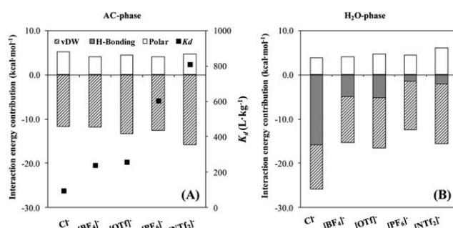
**Fig. 6** Predicted COSMO-RS contributions to interaction energies of (A) IL-AC and (B) IL-water for [C<sub>4</sub>C<sub>1</sub>im]<sup>+</sup> based ILs with Cl<sup>-</sup>, [BF<sub>4</sub>]<sup>-</sup>, [PF<sub>6</sub>]<sup>-</sup> and [NTf<sub>2</sub>]<sup>-</sup> anions.
