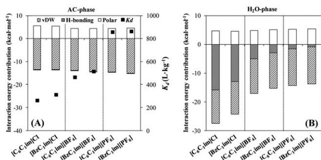
**Fig. 10** Predicted COSMO-RS contributions to interaction energies of (A) IL-AC and (B) IL-water for  $[C_6C_1\text{im}]^+$  or  $[\text{BzC}_1\text{im}]^+$  based ILs with  $\text{Cl}^-$ ,  $[\text{BF}_4]^-$  or  $[\text{PF}_6]^-$  anions.
