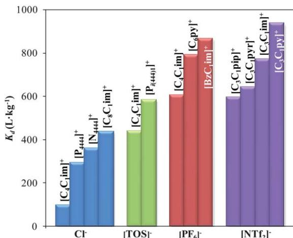
**Fig. 4** Comparison of  $K_d$  (obtained when  $C_e = 1.2 \text{ mmol L}^{-1}$  on AC-MkU at 308 K) for different ionic liquids.
