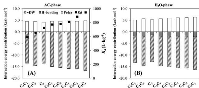
**Fig. 8** Predicted COSMO-RS contributions to interaction energies of IL-AC (A) and IL-water (B) for  $[C_nC_m\text{im}][\text{NTf}_2]$  based ILs with different alkyl chain substituents.
