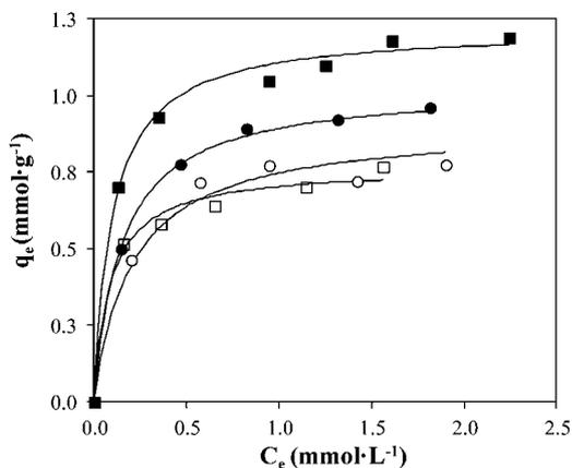
**Fig. 1** Experimental equilibrium data (dots) and Langmuir fits (curves) for the adsorption isotherms onto AC-MkU at 308 K of (□), [C<sub>3</sub>C<sub>1</sub>pip][NTf<sub>2</sub>]; (○), [C<sub>3</sub>C<sub>1</sub>pyr][NTf<sub>2</sub>]; (●), [C<sub>3</sub>C<sub>1</sub>im][NTf<sub>2</sub>] and (■), [C<sub>3</sub>C<sub>1</sub>py][NTf<sub>2</sub>].
