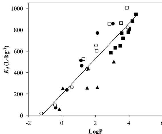
**Fig. 5** Experimental *K<sub>d</sub>* versus predicted log *P* by COSMO-RS for 32 ILs with a molecular volume below 0.4 nm<sup>3</sup> using AC-MkU as an adsorbent at 308 K: (■), [NTf<sub>2</sub>]<sup>-</sup>; (□), [PF<sub>6</sub>]<sup>-</sup>; (●), [BF<sub>4</sub>]<sup>-</sup> and (▲), others.
