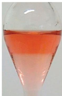
**Fig. 1** Macroscopic appearance of given ABS composed of an ionic liquid and an inorganic salt. Chloroanilic acid was added to colour (preferentially) the ionic-liquid-rich phase.
