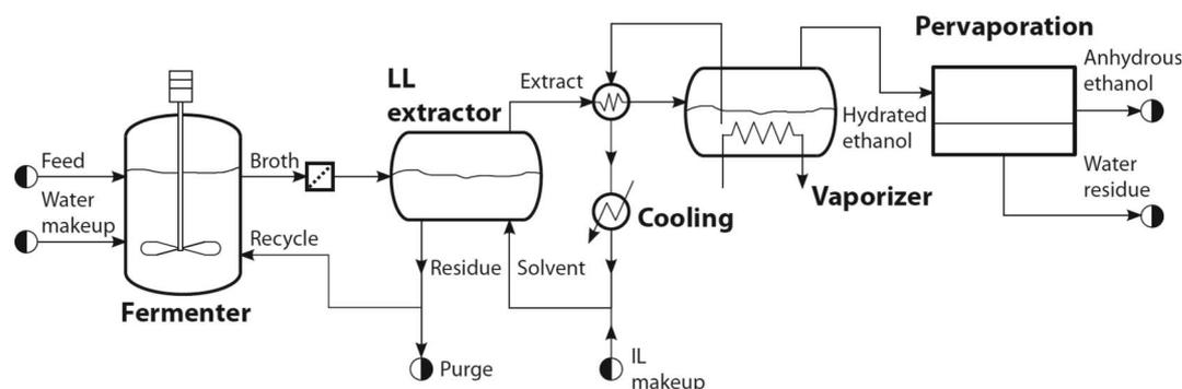
Fig. 10 Block diagram for ethanol purification based on liquid–liquid extraction and pervaporation.
