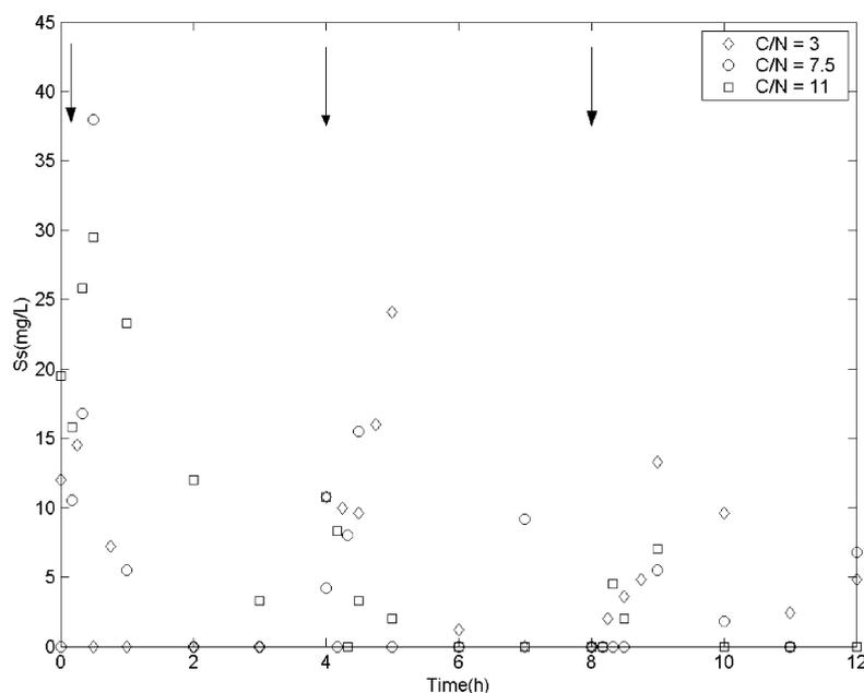
Fig. 4. Carbon oxidation data obtained for distinct  $C_{org}/N$  conditions in a SBR (arrows indicate initial feed step).
