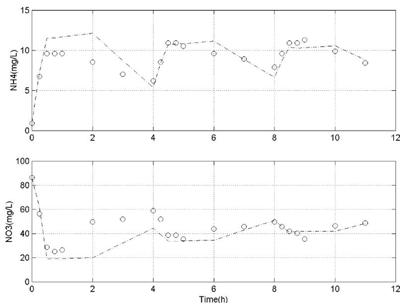
Fig. 6. Experimental data (○) and model prediction (---) for  $C_{\text{org}}/N$  ratio = 3.0.
