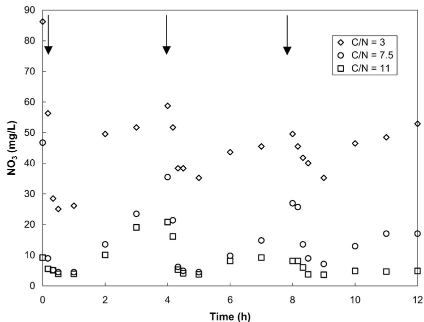
Fig. 3. Nitrate kinetic data obtained for distinct  $C_{org}/N$  conditions in a SBR (arrows indicate initial feed step).
