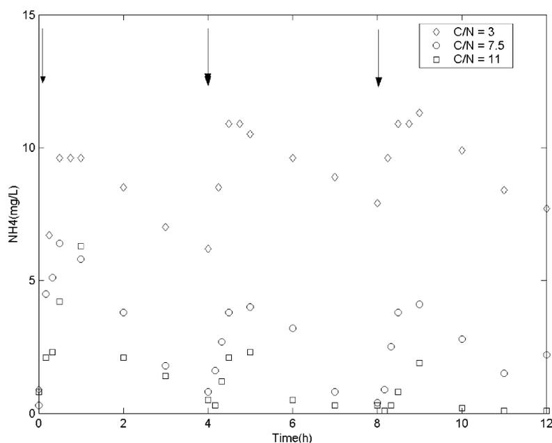
Fig. 2. Ammoniacal nitrogen kinetic data for distinct  $C_{\text{org}}/N$  conditions in a SBR (arrows indicate initial feed step).
