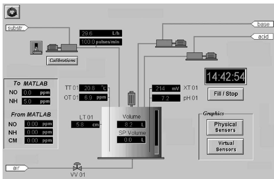
Fig. 1. Supervisory control: measurements and operation coordinates.
