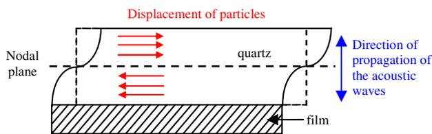
Figure 1. Shear waves in a quartz crystal.
