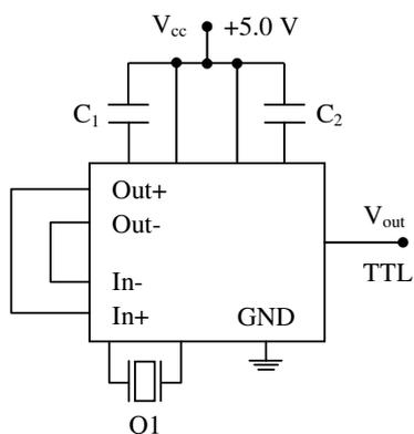
Figure 3. Schematic circuit of the crystal oscillator.
